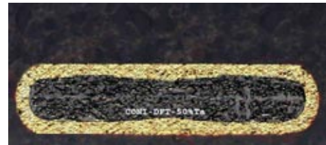
Figure 9: Flat DFT; Note: No interfacial separation after roll forming.
