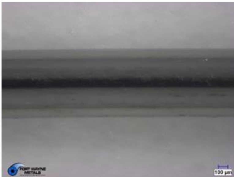
Figure 14. Alloy 420 As Drawn Surface
