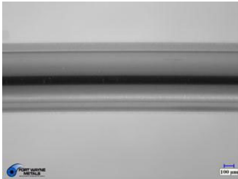
Figure 53. 35N LT® DFT®-41Ag Masked As Drawn Surface
