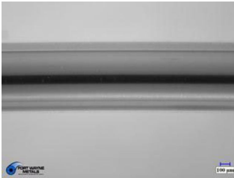
Figure 56. 35N LT® DFT®-41Ag Unmasked As Drawn Surface
