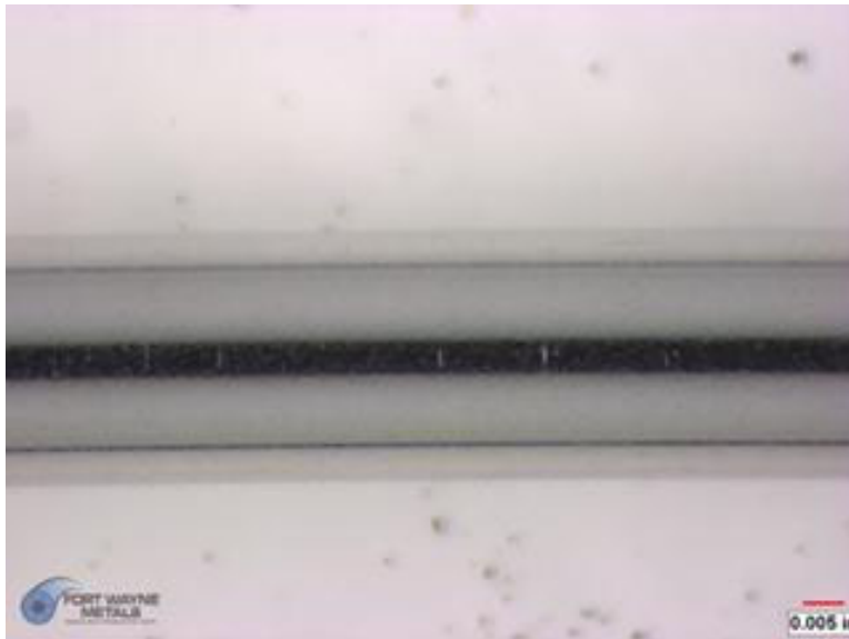
Figure 32. L605 Alloy As Drawn Surface
